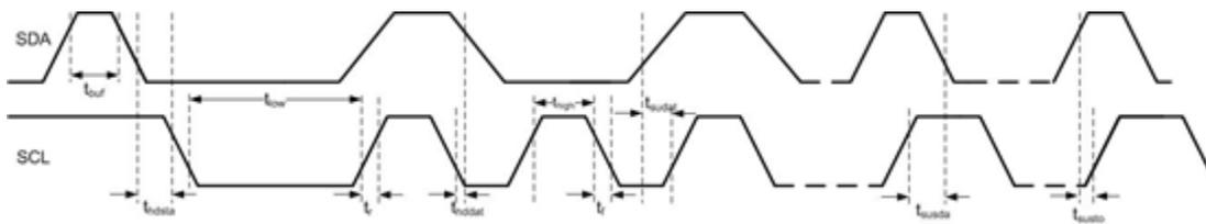
**Figure 11. I<sup>2</sup>C Timing Diagram**
