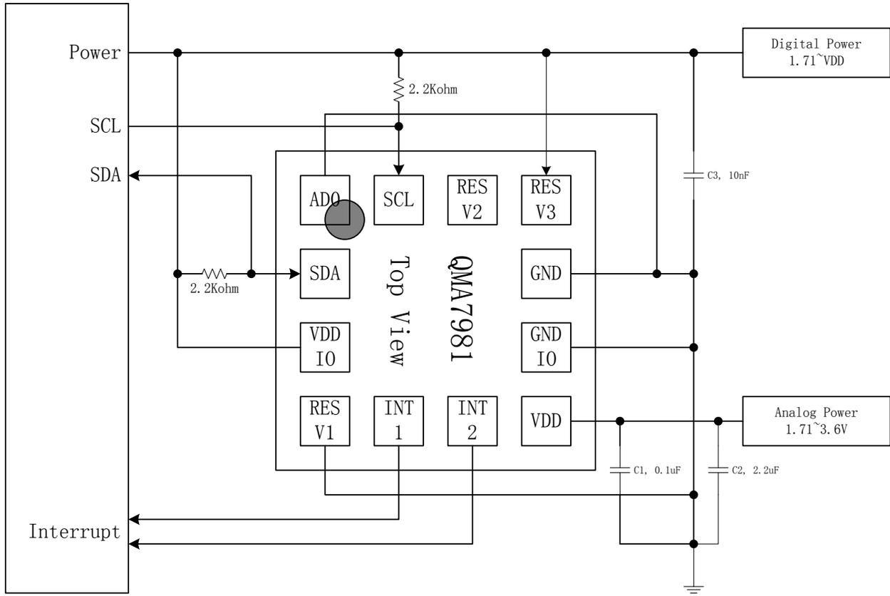
Figure 5. Dual Supply Connection
