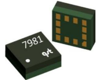
The QMA7981 is in a 2x2x0.95mm<sup>3</sup> surface mount 12-pin land grid array (LGA) package.
