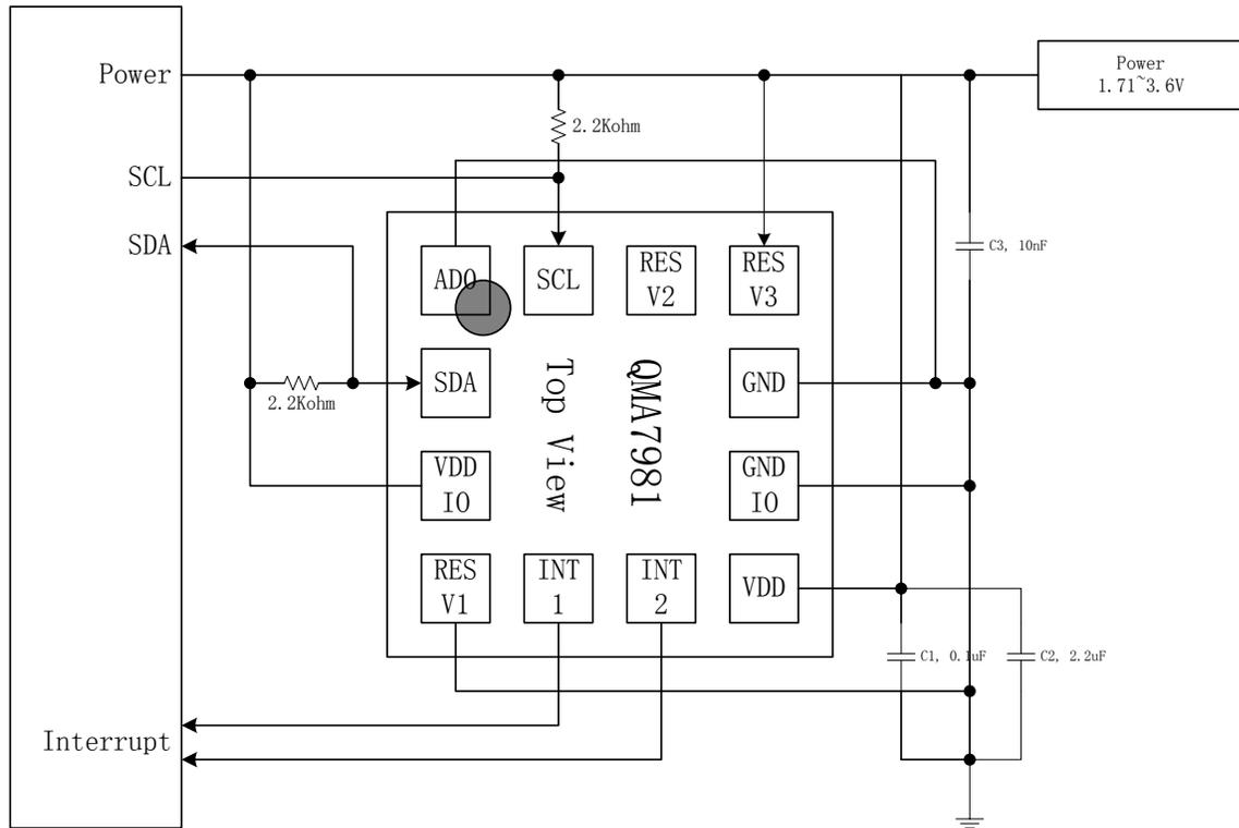
Figure 6. Single Supply Connection
